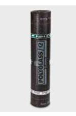
PLANA P is a prefabricated waterproofing elastomeric-plastomeric membrane, with a distilled bitumen-based compound modified with polypropylene and staple non-woven polyester fabric reinforcement. For use as a vapor barrier and as a provisional waterproofing measure to stop water getting in temporarily, it meets the requirements of standard EN 13970 and EN 13707.
