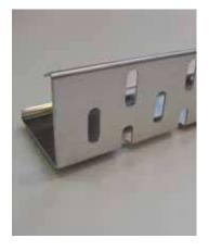
MAPEPLAN GRAVEL PROFILE is a separation and finishing profile for ballasted roofs with gravel or floating pavements, it is provided with oval holes to allow water drainage in frontal side and with oval eyelets for the anchorage with hot air welded strips on roofing membrane MAPEPLAN T.
