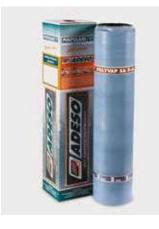
POLYVAP SA P-AL is a prefabricated double-sided self-adhesive bitumen membrane produced using ADESO technology, made up of a special selfadhesive elastomeric compound (SBS) reinforced with an aluminum foil. For use as a vapor barrier, it meets the requirements of standard EN 13970. Its use is recommended in all cases where application does not involve torching.
