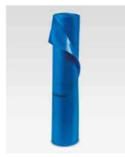
MAPEPLAN VB PE SD 220 is a synthetic sheet in polyethylene, of blue color, having a nominal thickness of 0,25 mm and  $S_d$  value of 220 m. It is used as vapor control layers and functional element for insulated roof build-ups, to be applied on the "warm side" of the thermal insulation
