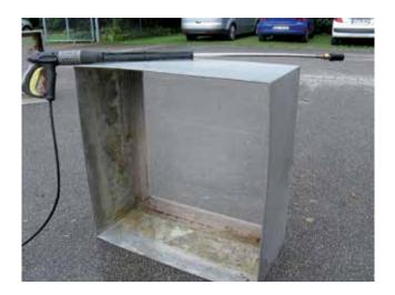
The bottom of the box is transparent, being made from Plexiglas, to allow for visual inspection at six-month intervals (to see whether roots have gone through the membrane). The test lasts for a total of two years, during which time visual inspections are carried out twice a year.
