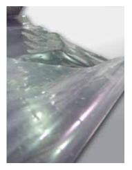
MAPEPLAN PE micro-perforated is an anti-soaking layer made from low-density polyethylene LDPE of transparent colour, with a nominal thickness of 0.10 mm and having a micro-perforation, which makes it permeable to vapour.
