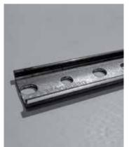
MAPEPLAN METALBAR is a metal fixing profile in galvanized carbon steel, prepunched, with oval perforations, to be used around the perimeter of the waterproofing membrane to anchor the sheet. Anti-tear cord MAPEPLAN T CORD is applied adjacent to the slotted profiles to complete the fastening of the perimeter.
