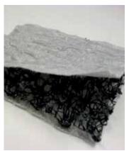
POLYSTUOIA 20 and POLYSTUOIA 20L are protective and drainage geocomposites comprising two UV-stabilized, needle-punched polypropylene staple-fibre filter geotextiles with a 3-dimensional drainage structure sandwiched between them made up of polypropylene monofilaments. The two geotextiles are heat bonded to the drainage core using a continuous process.
