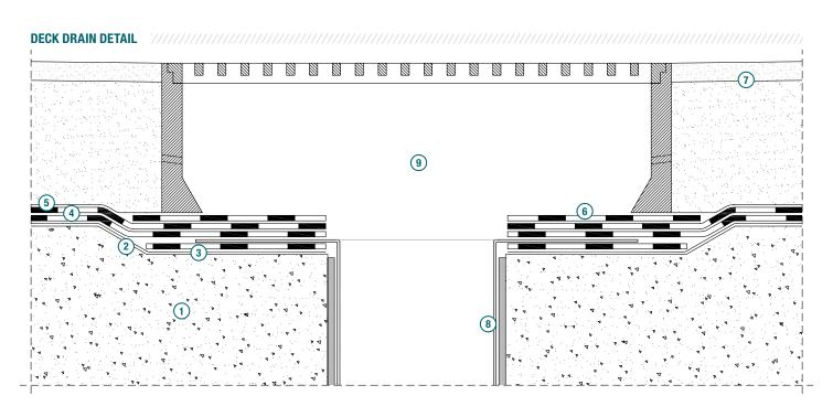
1. Substrate - Reinforced concrete slab - 2. POLYPRIMER HP 45 Professional or IDROPRIMER bituminous primers - 3. POLYGLASS reinforcing waterproofing membrane - 4. POLYGLASS deck waterproofing membrane (first layer) - 5. POLYGLASS deck waterproofing membrane (second layer) - 6. POLYGLASS protective waterproofing membrane - 7. Road surfacing - Binder course and wearing course per design - 8. Outlet - 9. Frame and grate suitable for vehicle traffic.
