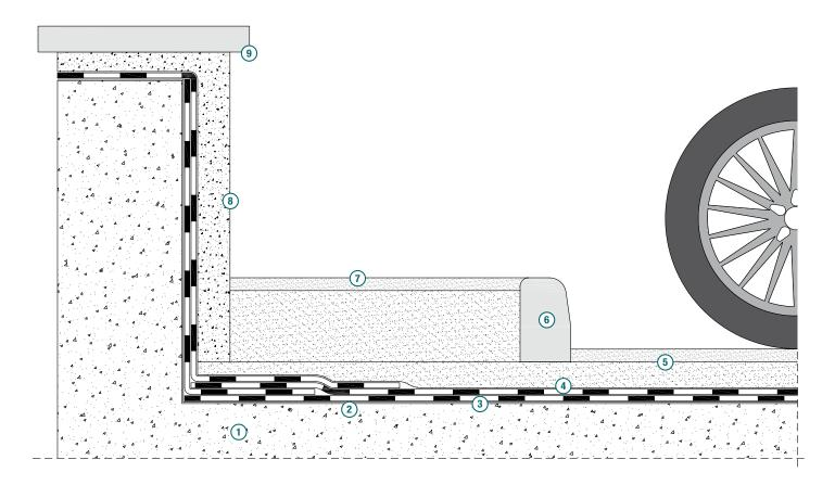
1. Substrate - Reinforced concrete slab - 2. POLYPRIMER HP 45 Professional or IDROPRIMER bituminous primers - 3. POLYGLASS deck waterproofing membrane (first layer) - 4. POLYGLASS deck waterproofing membrane (second layer) - 5. Road surfacing - Binder course and wearing course per design - 6. Protective kerb - 7. Pavement - 8. Turn-up protected with mesh and plaster - 9. Finishing detail.
