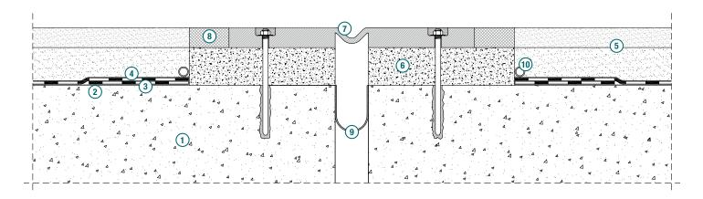
1. Substrate - Reinforced concrete slab - 2. POLYPRIMER HP 45 Professional or IDROPRIMER bituminous primers or EPOXY PRIMER - 3. POLYGLASS SBS reinforcing membrane - 4. POLYGLASS bridge waterproofing membrane (type: POLYBOND HP, POLYFLEX HP, ELASTOFLEX HP, EVOLIGHT HP or POLYFLEX LIGHT HP) - 5. Road surfacing - Binder course and wearing course per design - 6. Mortar bedding - 7. Expansion joint - 8. Infill mortar acting as a buffer - 9. Flashing - 10. Drainage pipe.
