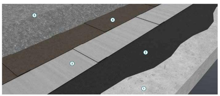
**1.** Substrate - Reinforced concrete slab - **2.** POLYPRIMER HP 45 Professional or IDROPRIMER bituminous primers - **3.** POLYGLASS deck waterproofing membrane (first layer) - recommended thickness: 5 mm - **4.** POLYGLASS deck waterproofing membrane (second layer) - recommended thickness: 4 mm - **5.** Road surfacing - Binder course and wearing course per design.
