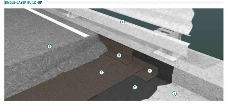
1. Substrate - Reinforced concrete slab - 2. POLYPRIMER HP 45 Professional or IDROPRIMER bituminous primers or EPOXY PRIMER - 3. POLYGLASS bridge waterproofing membrane (type: POLYBOND HP, POLYFLEX HP, ELASTOFLEX HP, EVOLIGHT HP or POLYFLEX HP LIGHT -recommended thickness: 5 mm) - 4. Reinforced strip with POLYGLASS waterproofing membrane - 5. Vertical turn-up with POLYGLASS bridge waterproofing membrane 6. Road surfacing - Binder course and wearing course per design - 7. Guardrail
