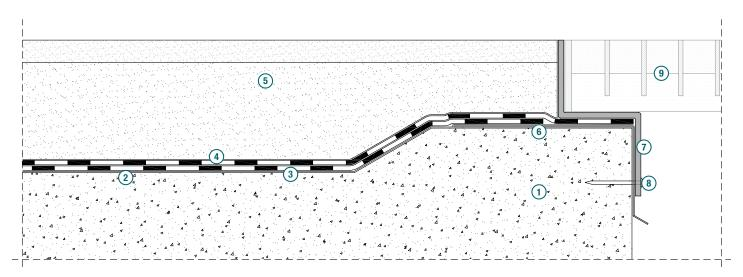
1. Substrate - Reinforced concrete slab - 2. POLYPRIMER HP 45 Professional or IDROPRIMER bituminous primers - 3. POLYGLASS deck waterproofing membrane (first layer) - 4. POLYGLASS deck waterproofing membrane (second layer) - 5. Road surfacing - Binder course and wearing course per design - 6. Lower flashing - 7. Upper flashing in stainless steel or galvanized steel **8.** Mechanical fixing - **9.** Metal grate suitable for vehicle/pedestrian traffic.
