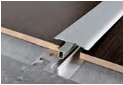
ALU. TOP + PIN INSERT + ALU. BASE 45 PUNCHED/PERFORATED (6 anod. al. finishes of which 3 on demand) thermo packed bar length 2,7 LM - pack. 20 Pcs - 54 LM (H 17 - 19mm - 40,5 LM)
